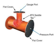
Vacuum tested to a maximum of 30 in. water column with no leakage at seal to tap. Pressure tested to a maximum of 39 PSI with leakage at tap seal (see chart below)
