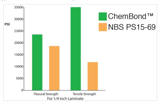
For structural tests, samples were sent to California State University at Long Beach. CSULB determined the tensile strength, flexural modulus, and the flexural strength for a laminate of ChemBond™ resin and glass reinforcement. These values were considerably greater than those recommended in the National Bureau of Standards Product Standard 15-69.
