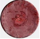
After exposure to 96% Sulfuric acid for 31 days at 39°C (102°F)
