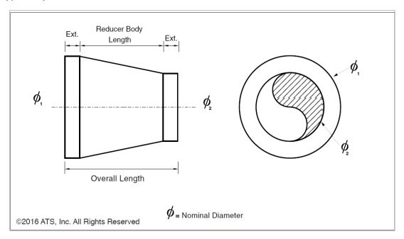
ATS special length reducers are designed to meet conditions at the job site where standard length reducers (5 to 1 - length to reduction in diameter) will not suffice. Customer to specify the overall length along with the diameter change.
