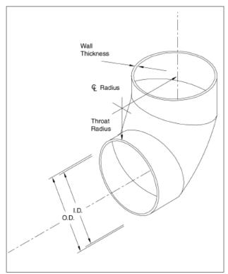
ATS 90° 3 gore mitered elbows are made to customer specifications. Part type #24 is ideal for applications where tight turning radii or other limitations on size and space make using standard sweep radius elbows impossible.
