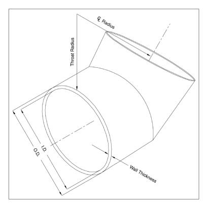
ATS 45° 2 gore mitered elbows are made to customer specifications. This part is ideal for applications where tight turning radii or other size/space limitations make using standard sweep radius elbows impossible. The use of ATS gored elbows allows for design and installation flexibility.
