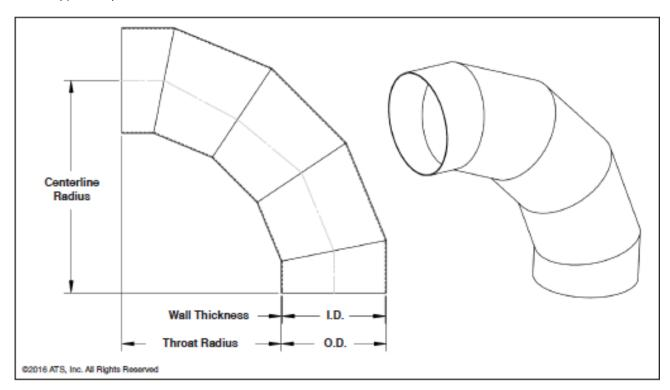
ATS 90° 5 gore mitered elbows are made to customer specifications. Part type #25 is used for better airflow. 5 gore mitered elbows available in any standard nominal diameter.
